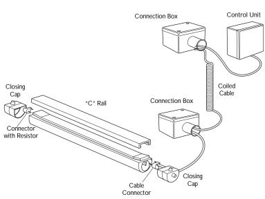
Example application of profile using coiled cable. The coiled cable can not be directly connected to the profile due to the weight of the cable. The proper use of the coiled cable is to connect the coiled cable to the profile through the connection box. The coiled cable should be secured to both the moving and stationary objects so as to prevent straining of the terminal connections.
