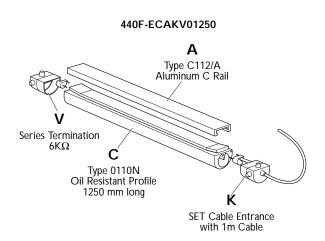
This is a single oil resistant profile which is 1250mm long. The edge is terminated with a Series Termination. A 1m cable enters straight into the closing cap from a DIN-rail mounted controller. The profile is mounted on a standard aluminium C rail.
